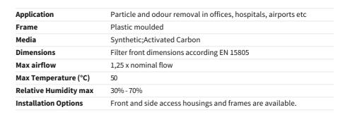
A compact filter with an additional molecular filtration media layer to provide enhanced IAQ through combined particle filtration and gas filtration.
